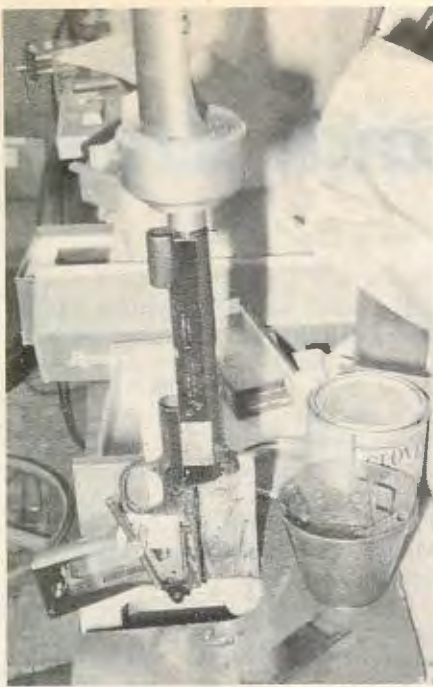
Above: Slide and Frame are then lapped in special machine to insure fit and minimize galling and wear.
